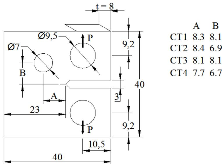
Figure 7 Geometry of the modified CT specimens (dimensions in mm)
