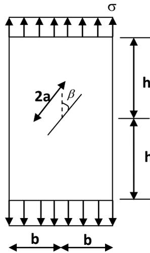
Figure 4 Inclined central crack in rectangular plate under monotonic loading
