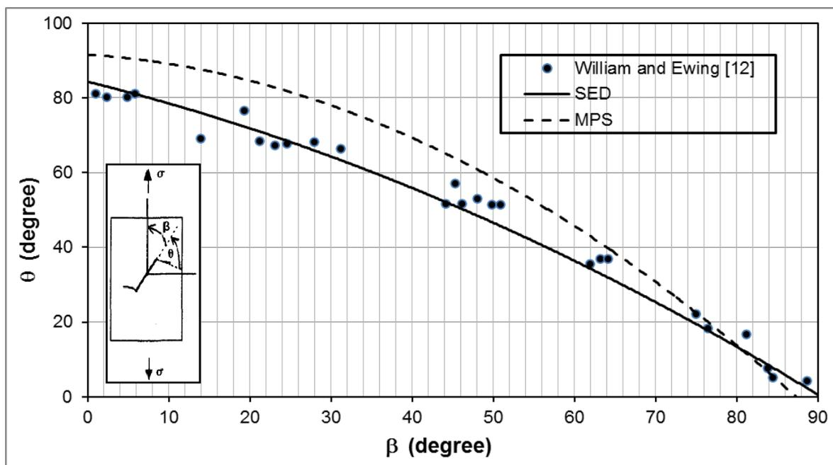
Figure 6 Comparison between FEM from SED and MPS criteria and experimental data [12] for inclined central crack plate under monotonic loading.
