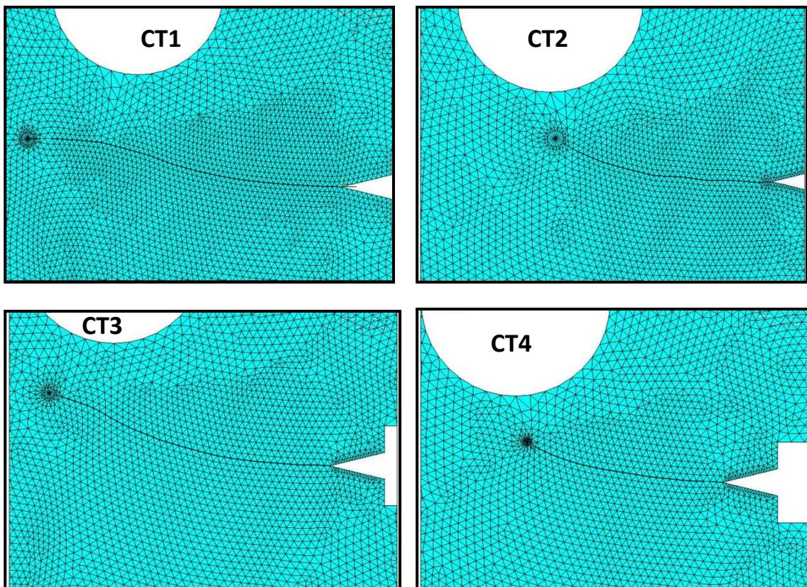
Figure 8 FE meshes automatically generated for modified CT specimens
