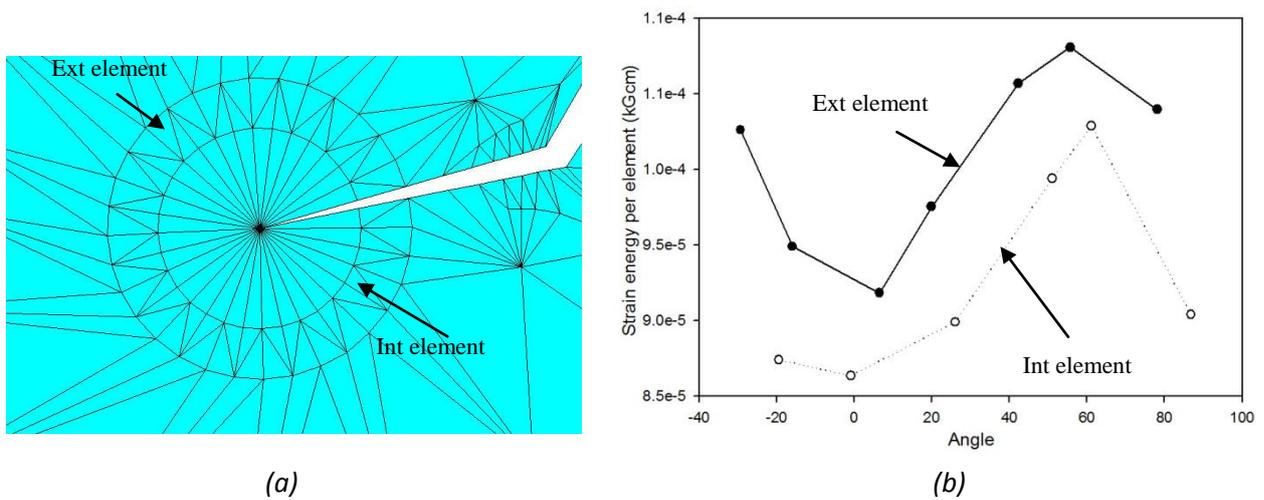
Figure 2 (a) Ring elements around crack tip; (b)  $S(\theta)$  curve
