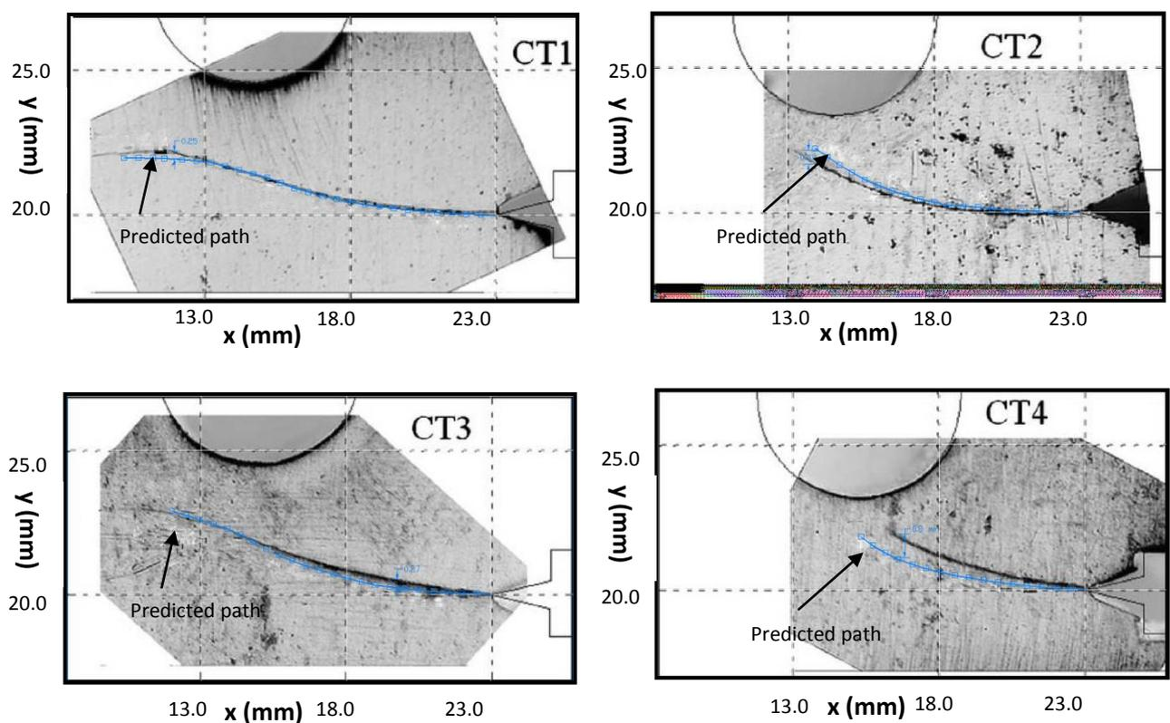
Figure 9 Comparison between predicted and measured [15] crack paths for modified CT specimens.
