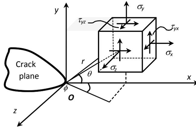
Figure 1. Stress components in element around crack tip
