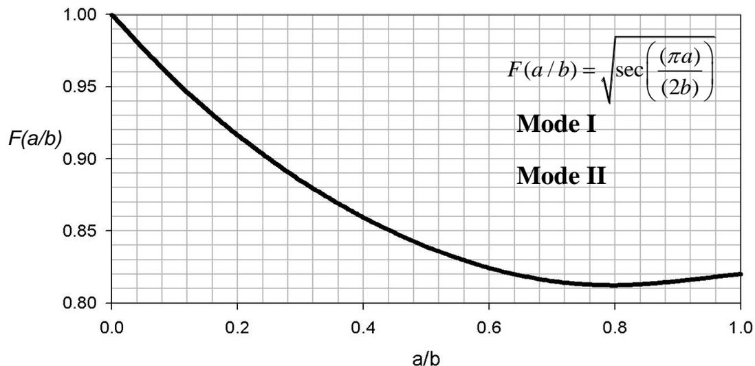
Figure 5  $F(a/b)$  for Mode I and Mode II (Tada et al. [13])
