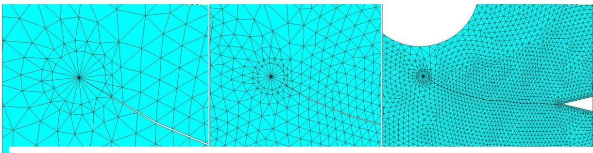
Figure 3 Evolutionary mesh refinement at the tip as the crack propagates
