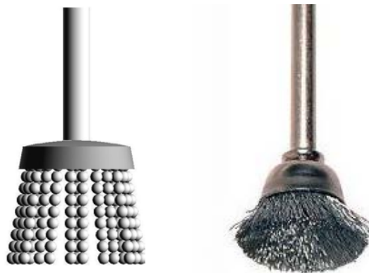
Figure 3. Small cup brush model (left) and real cup brush (right)
