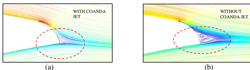
Figure 11. Flow Fields of S809 airfoil (a) with, and (b) without - Coandă -jet
