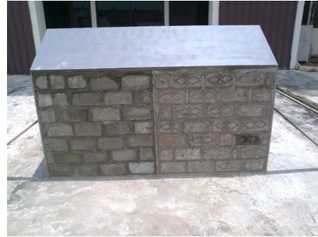
Figure 3. Conventional concrete block (right) and concrete block with MEPCM (left)
