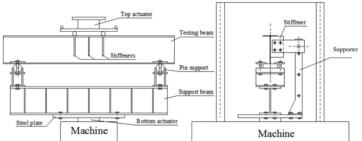
Figure 1. Schematic of testing system
