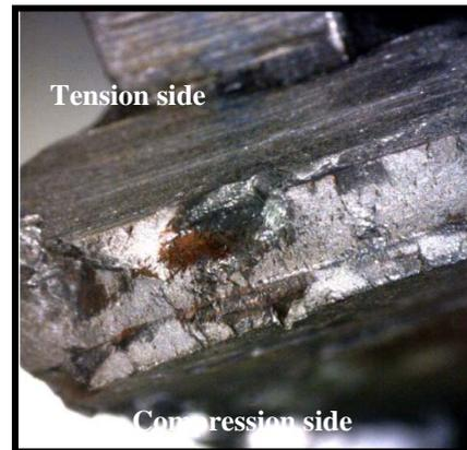
(A) Initiation of the first crack at weld toe
