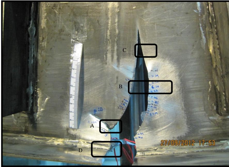
Figure 9. Pictures of the first and second cracks
