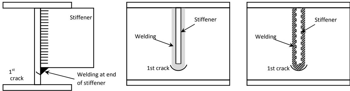
Figure 6. Crack propagation in stage 1
