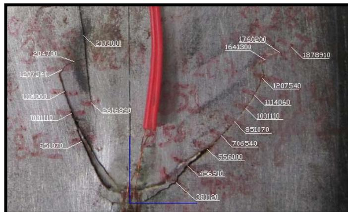
Figure 11. Recorded fatigue life on specimen
