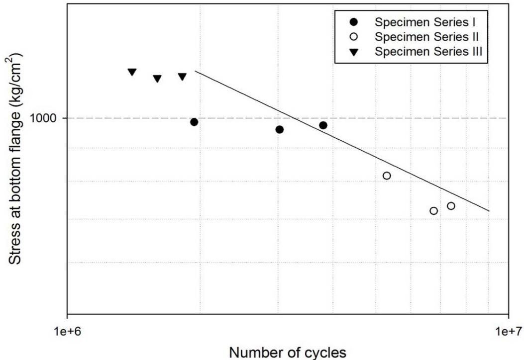
Figure 12. S-N curve from the test data
