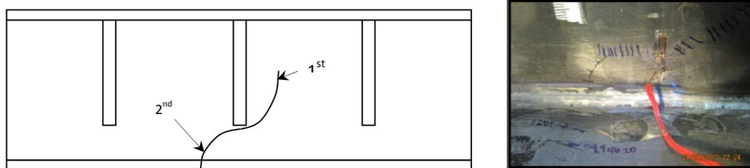
Figure 5. Specimen failures due to initial crack going downward
