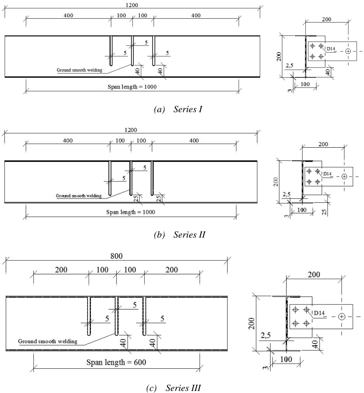
Figure 2. Dimensions of three series of specimens
