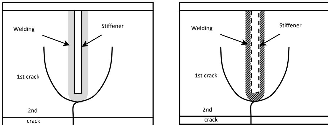
Figure 8. Crack propagation in stage 3
