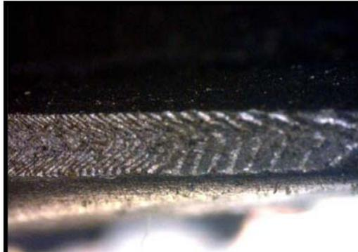
(B) Propagation of the first crack
