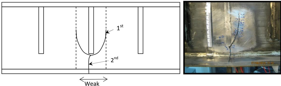
Figure 3. Specimen failure due to new crack in “weak zone”
