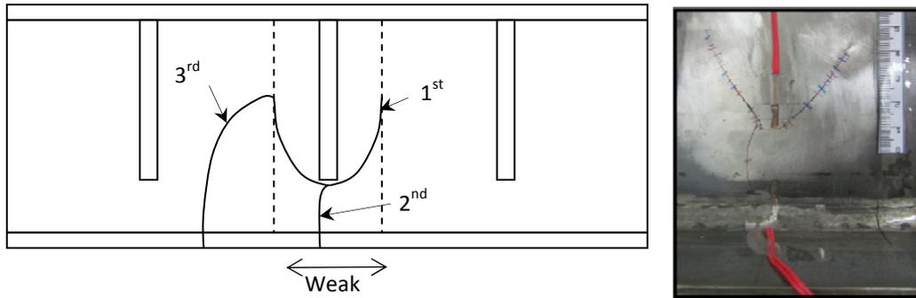
Figure 4. Specimen failure due to new crack occurring outside “weak zone”
