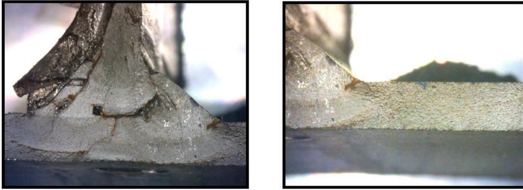
(D) Propagation of the critical second crack to the bottom flange
