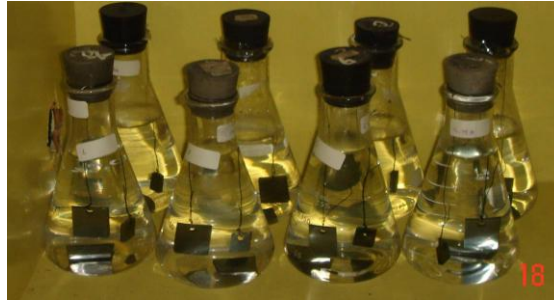
Figure 1. Immersion of steel samples in the media
