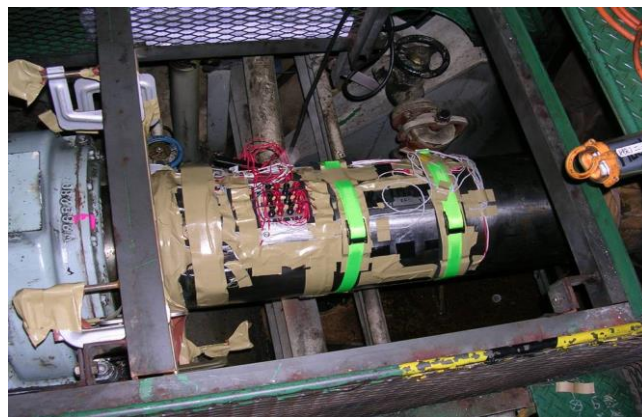
Figure 6. Strain gauges were attaching on propeller shaft
