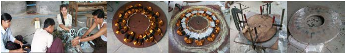
Figure 2. Stator coils casting from the mould
