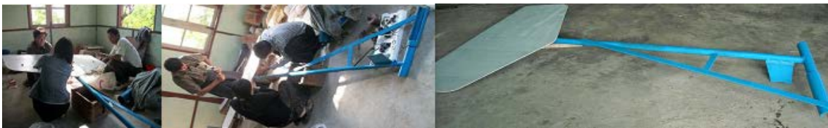
Figure 6. Tail vane bolted to the tail boom
