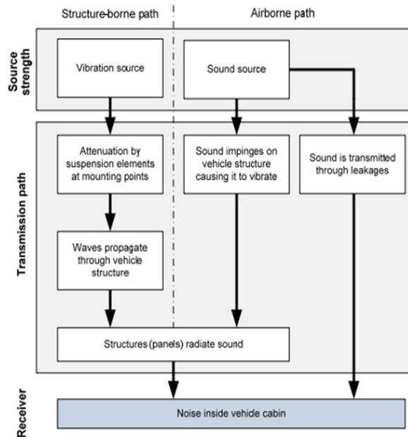
Figure 1. Vehicle interior noise transmission path [4]
