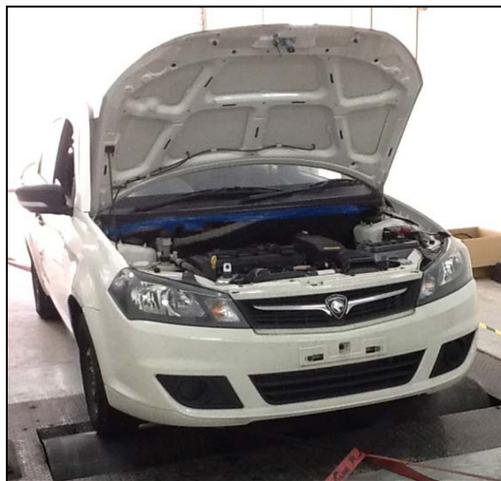
Figure 4. Test vehicle running on dynamomete
