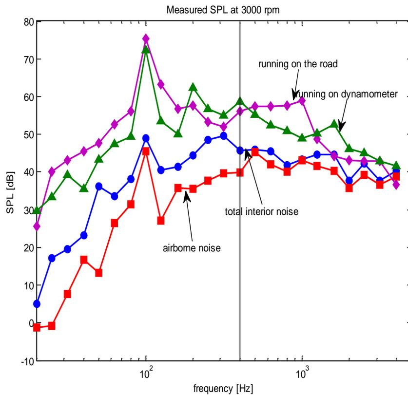
Figure 16. Combined SPL (stationary and running on road + on dynamometer) at 3000 rpm
