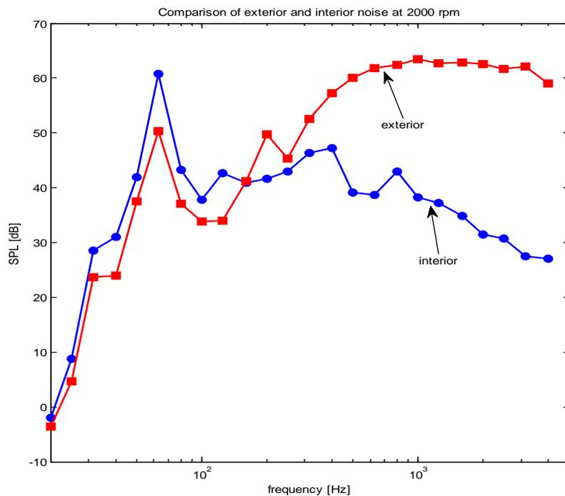
Figure 6. Measured SPL when engine is running at 2000 rpm
