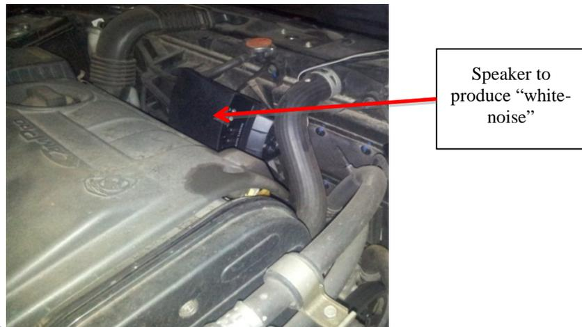
Figure 3. Location of the loudspeaker for exterior noise measurement using substitution source
