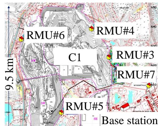
Figure 2. Rain gauge stations installed at different locations in Mae Moh coal lignite mine
