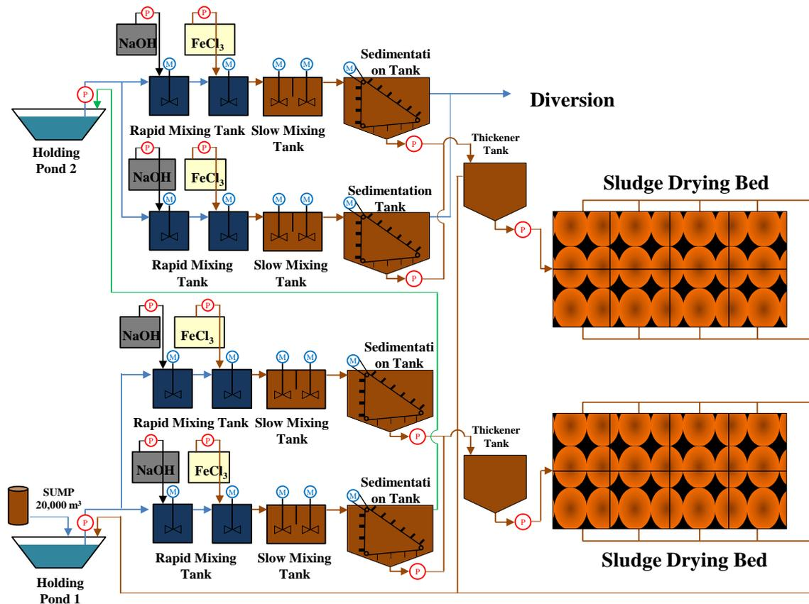
Figure 18. Flow diagram of water treatment plant of Mae Moh lignite mine (as of 2013) (Reproduced from the chart of Mine Environmental Management Department, EGAT)
