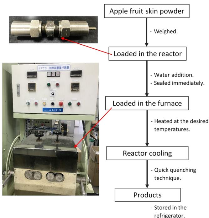
Figure 2 Extraction procedure by subcritical water
