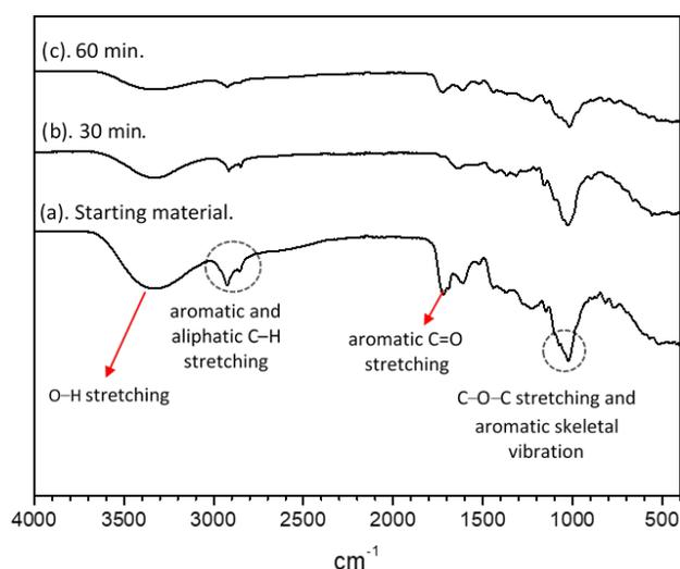
**Figure 3** FT-IR spectrum of apple fruit skin (starting material and its solid residue)
