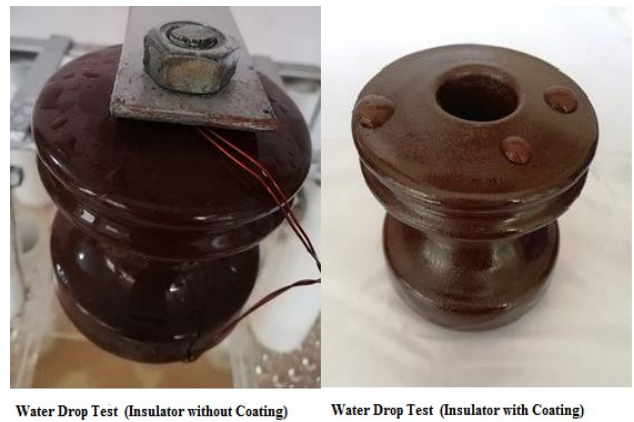
Figure 8 Water drop test on coated and uncoated insulators
