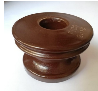
Figure 6 Insulator after applying Hydrophobic coating
