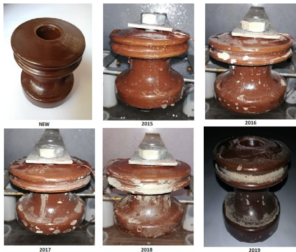
Figure 7 Accelerated aging of coated insulator as per coastal area weather condition
