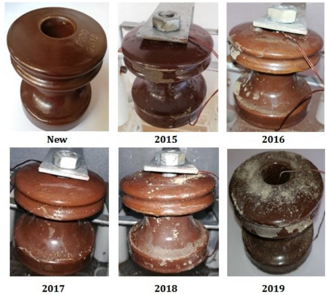
Figure 5 Accelerated aging of uncoated insulator as per coastal area weather condition
