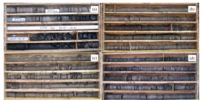
Figure 10 Photos of cores collected from NED-02A Borehole (a) cores at 63-68 m depth (b) cores at 148-153 m depth (c) cores at 204-209 m depth (d) cores at 280-285 m depth
