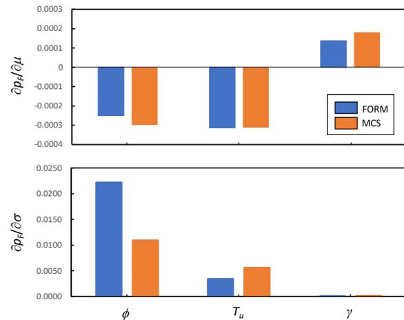
Figure 7 Comparison of reliability-based sensitivities calculated with FORM and Monte Carlo simulation (MCS) for MSE wall height  $H = 2.5$  m, layer spacing  $s_v = 0.2$  m, and effective tensile capacity factor  $R = 0.75$
