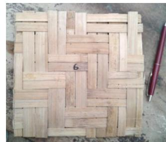
**Figure 2** Specimen of woven bamboo mat (WBM)
