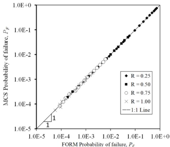
**Figure 9** Plots of  $p_F$  calculated with FORM against Monte Carlo simulation (MCS) for various MSE wall heights and effective tensile capacity factors
