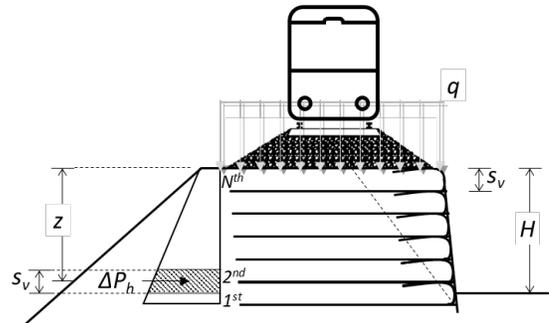
Figure 3 Design section of MSE wall for temporary railway embankment
