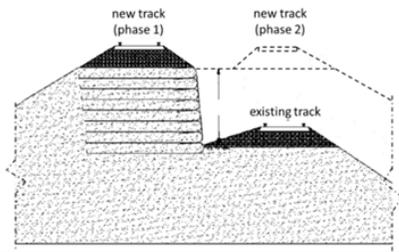
**Figure 1** The construction phase of Purwokerto-Kroya double track
