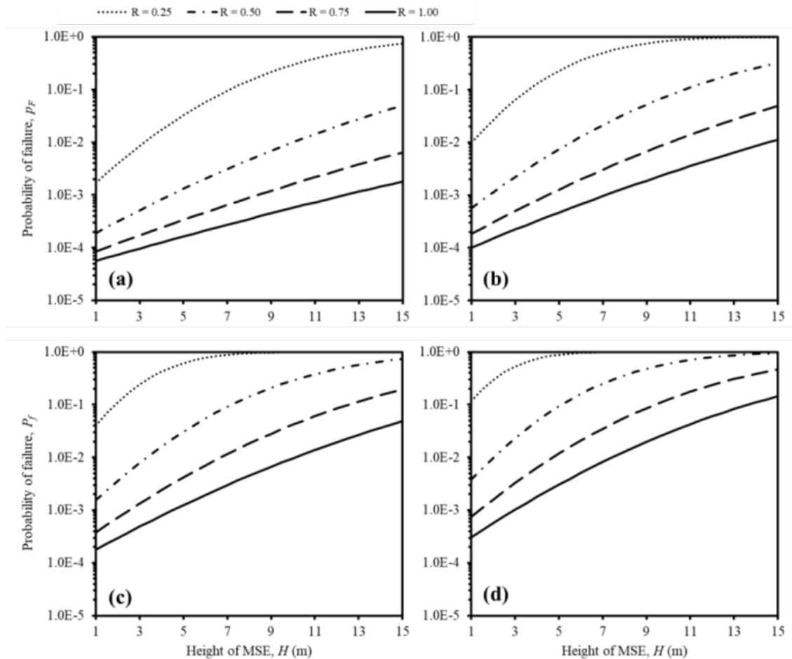
**Figure 8** Plot of height of MSE,  $H$  against probability of failure,  $p_F$ . (a)  $s_v = 0.2$  m; (b)  $s_v = 0.3$  m; (c)  $s_v = 0.4$  m; (d)  $s_v = 0.5$  m.
