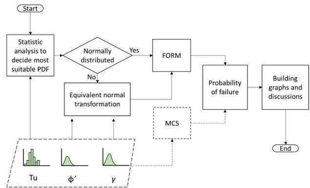
**Figure 4** Framework of reliability-based assessment of WBM MSE
