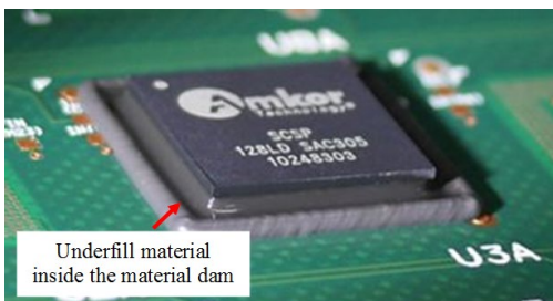
Figure 8 Underfill Material – Underfill inside the material dam
