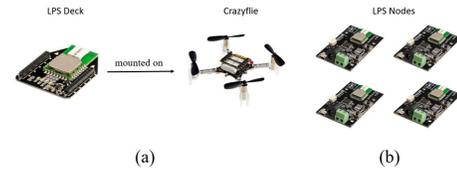
Figure 9 (a) Loco Positioning Deck to be mounted on Crazyflie, (b) Loco Positioning Nodes, images adapted from [14,19-20]
