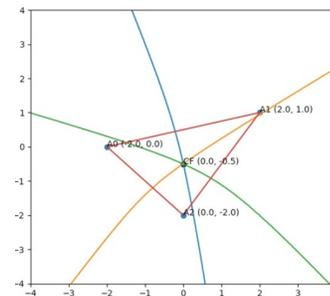
Figure 2 Aerial Drone Estimation with 3 Anchors, adapted from [18]
