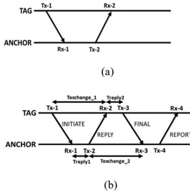
Figure 1 (a) TWR for 2 Message Packets (b) TWR Protocol
