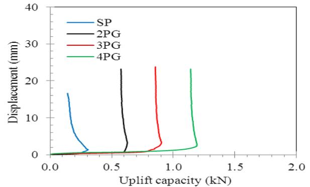
Figure 9 Uplift capacity for the pile group versus settlement under different the pile number in a group
