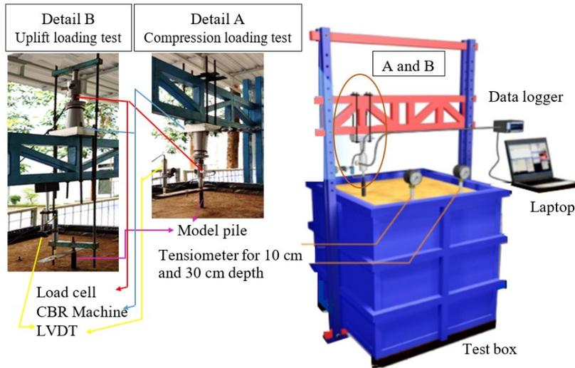
Figure 2 Setups of model piles for compression and uplift loading tests [18]
