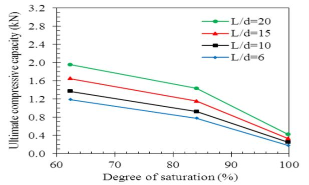
Figure 8 Ultimate compressive capacity for single pile versus degree of saturation of soil under different  $L/d$  ratio.
