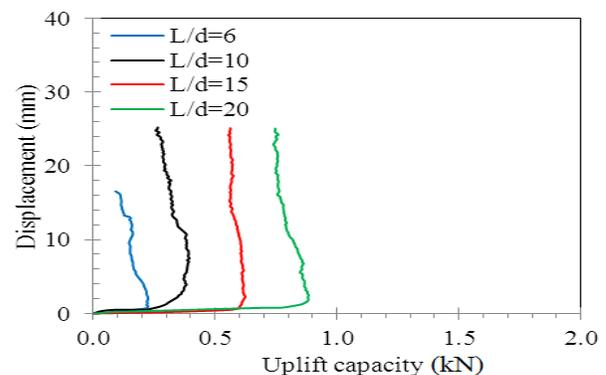
Figure 5 Single pile uplift capacity versus displacement under the different ratio of  $L/d$
