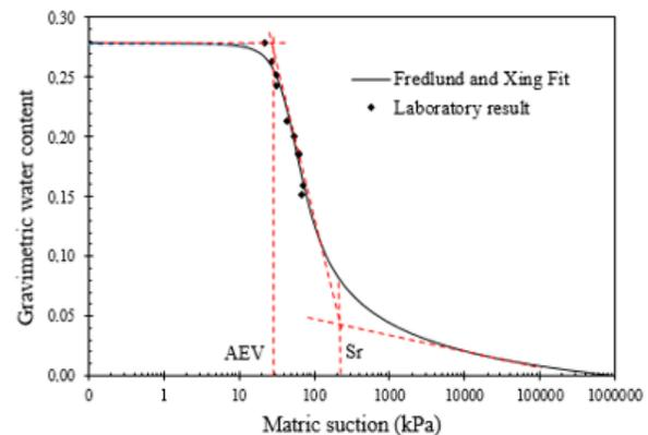
Figure 1 The hydromechanical behavior of sandy clay
