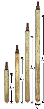
Figure 3 Single pile models:  $L_1= 96$  mm;  $L_2= 160$  mm;  $L_3= 240$  mm;  $L_4= 320$  mm,  $d= 16$  mm
