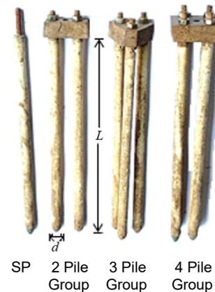
Figure 4 Group pile models:  $L= 200$  mm;  $d= 10$  mm
