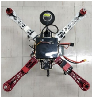
Figure 5 Local FC mounted on F450 frame
