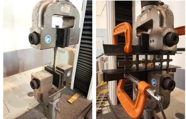
Figure 7 Left image: Tensile test of plastic mixtures by the Single-rib Method; Right image: Tensile test of plastic mixtures by the Multi-rib Method
