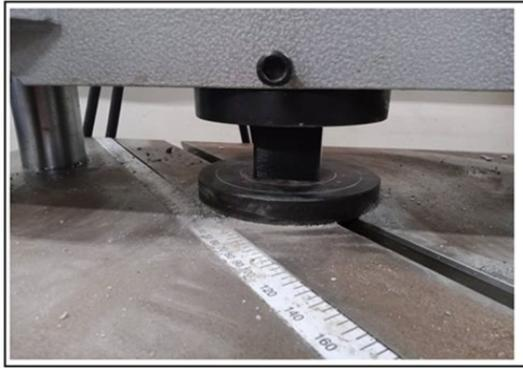
Figure 9 Compressive Test using UTM
