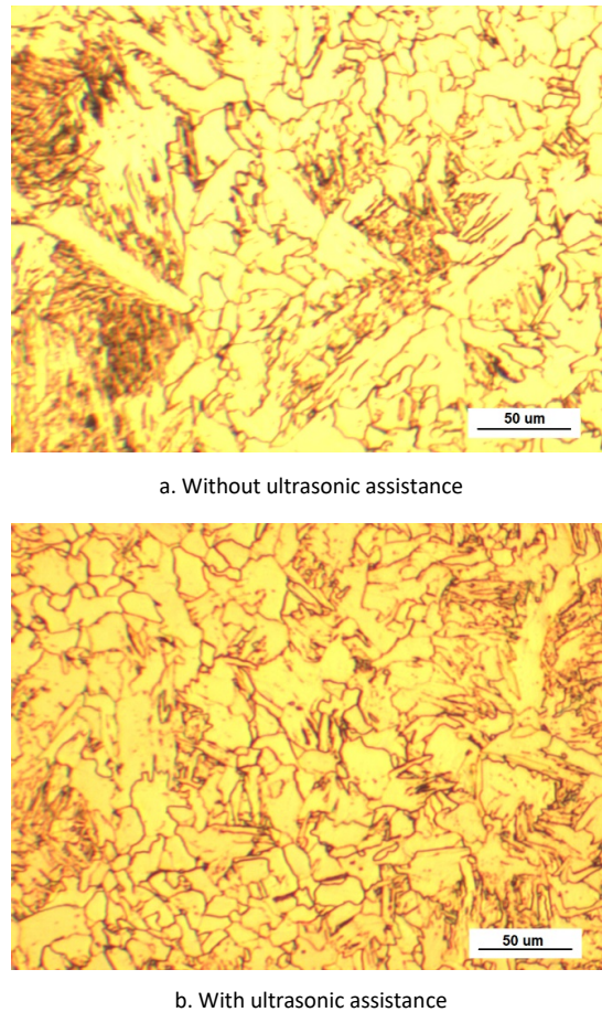
Figure 5 The microstructure of the fusion zone of the welded samples
