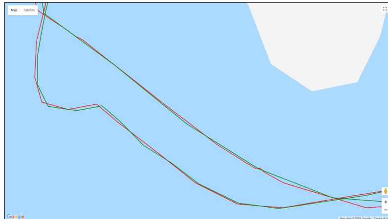
Figure 18. Tracking data during a boat ride. Green track represents the tracking device and the red track represents data from a commercial global positioning system (GPS) logger
