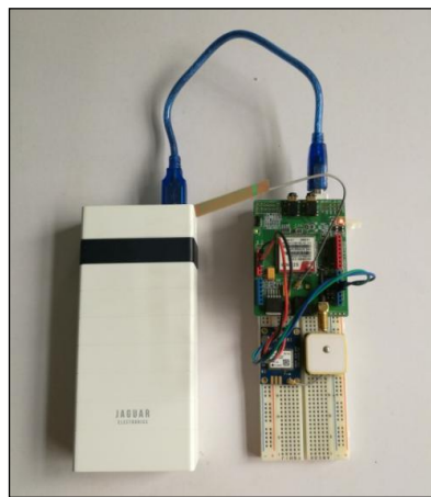
Figure 6. The tracking system device hardware
