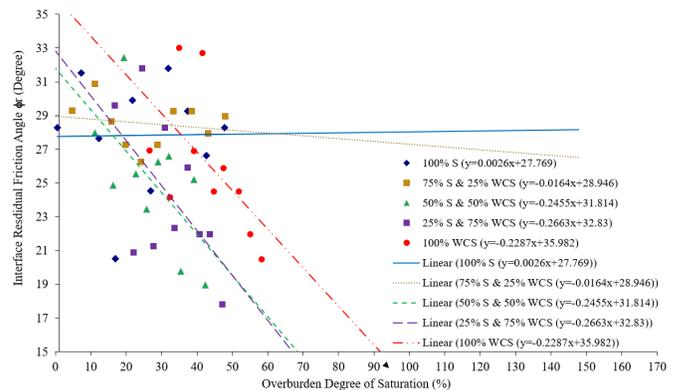
Figure 5 Interface friction angle for all variations
