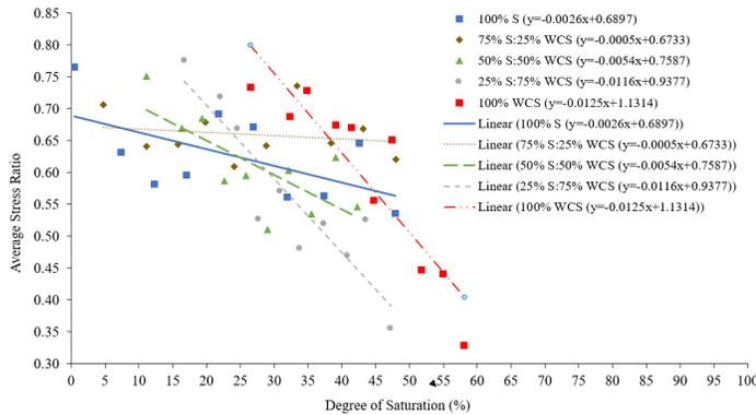
Figure 6 Average stress ratio for overburden degree of saturation of all variations
