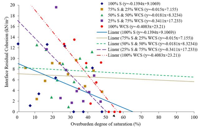
Figure 4 Interface cohesion for all overburden layers
