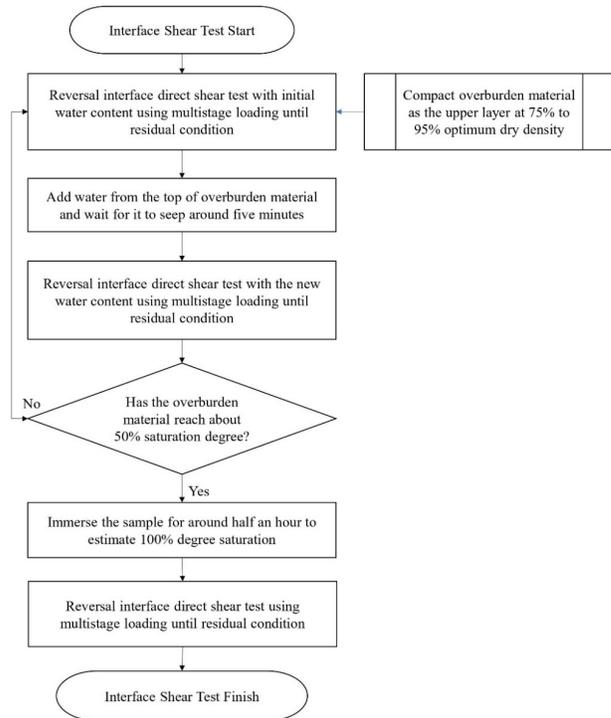
Figure 1 Interface Shear Test Flowchart
