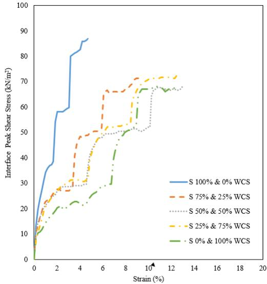
Figure 2 Peak Shear-Strain Graph for All Overburden Variations
