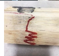
Figure 11. Splintering tension failure mode
