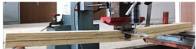
Figure 10. Simple tension failure mode
