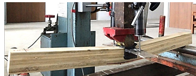
Figure 10. Simple tension failure mode
