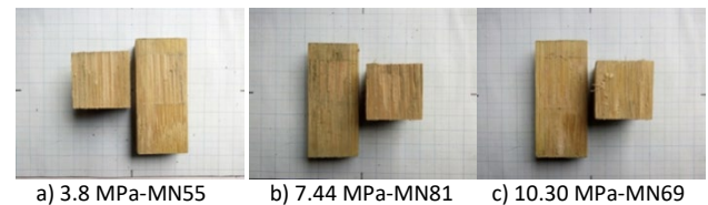
Figure 5. glue line shear failure of the MD block sample of the untreated LBL (adhesive bonding strength-sample code)
