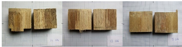
a) 4.57 MPa-AN66 b) 7.52 MPa-AN59 c) 10.04 MPa-AN43 Figure 7. glue line shear failure of the ASTM D905 sample of the untreated LBL (adhesive bonding strength-sample code)
