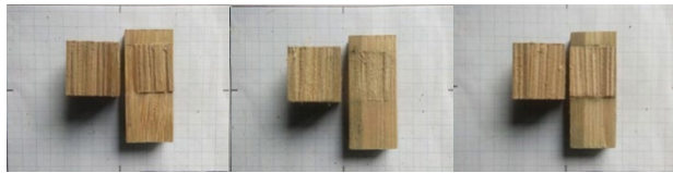
a) 3.45 MPa-MA79 b) 7.08 MPa-MA43 c) 10.47 MPa-MA17 Figure 6. glue line shear failure of the MD block sample of the treated LBL (adhesive bonding strength-sample code)
