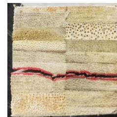
Figure 12. Horizontal shear (bamboo failure) failure mode
