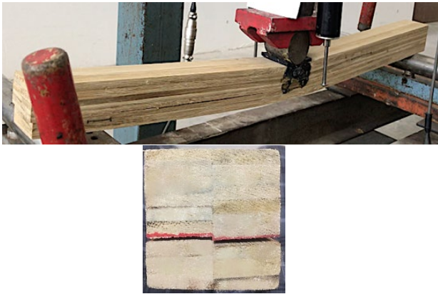
Figure 13. Horizontal shear (delamination) failure mode
