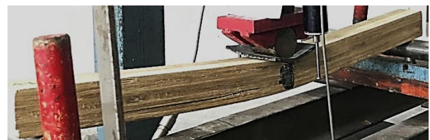
Figure 11. Splintering tension failure mode
