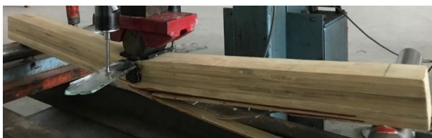
Figure 14. Simple tension & Horizontal shear but not delaminated failure mode
