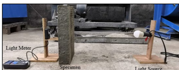
The 6 × 6 grid configurations of LTC under light transmittance test
