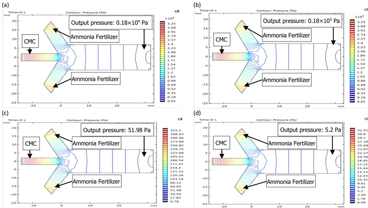
Figure 5 Output pressure for flow rate (a) 1 g/s , (b) 0.1 g/s , (c) 0.01 g/s and (d) 0.001 g/s in tri-axial milli-fluidic
