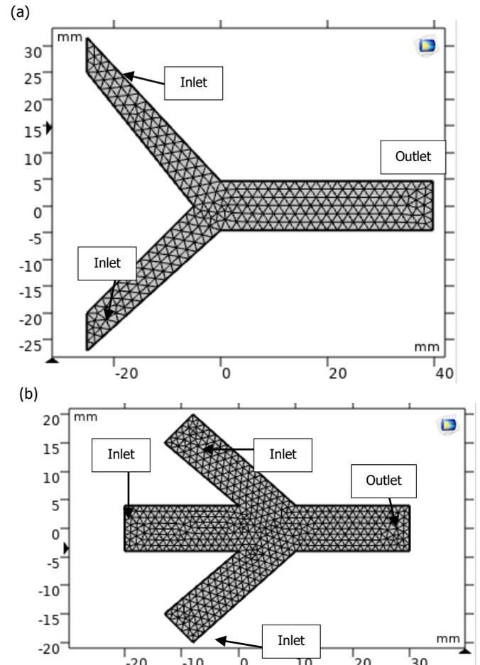
**Figure 2** The finite elements mesh of (a) co- and (b) tri-axial milli-fluidics
