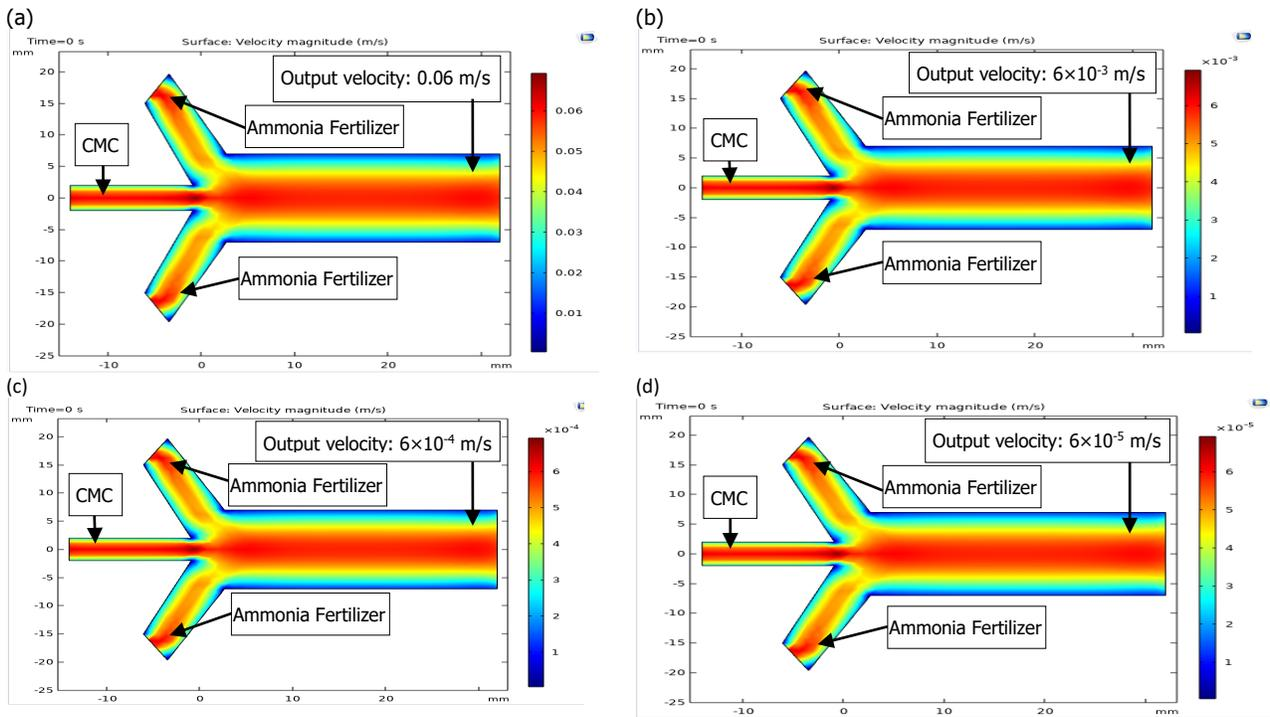
Figure 4 Output velocity for flow rate (a) 1 g/s , (b) 0.1 g/s , (c) 0.01 g/s and (d) 0.001 g/s in tri-axial milli-fluidic
