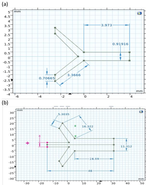
**Figure 1** The constitutive two-dimensional models of the (a) co- and (b) tri-axial milli-fluidic designed for co-linear extrusions of fertilizer
