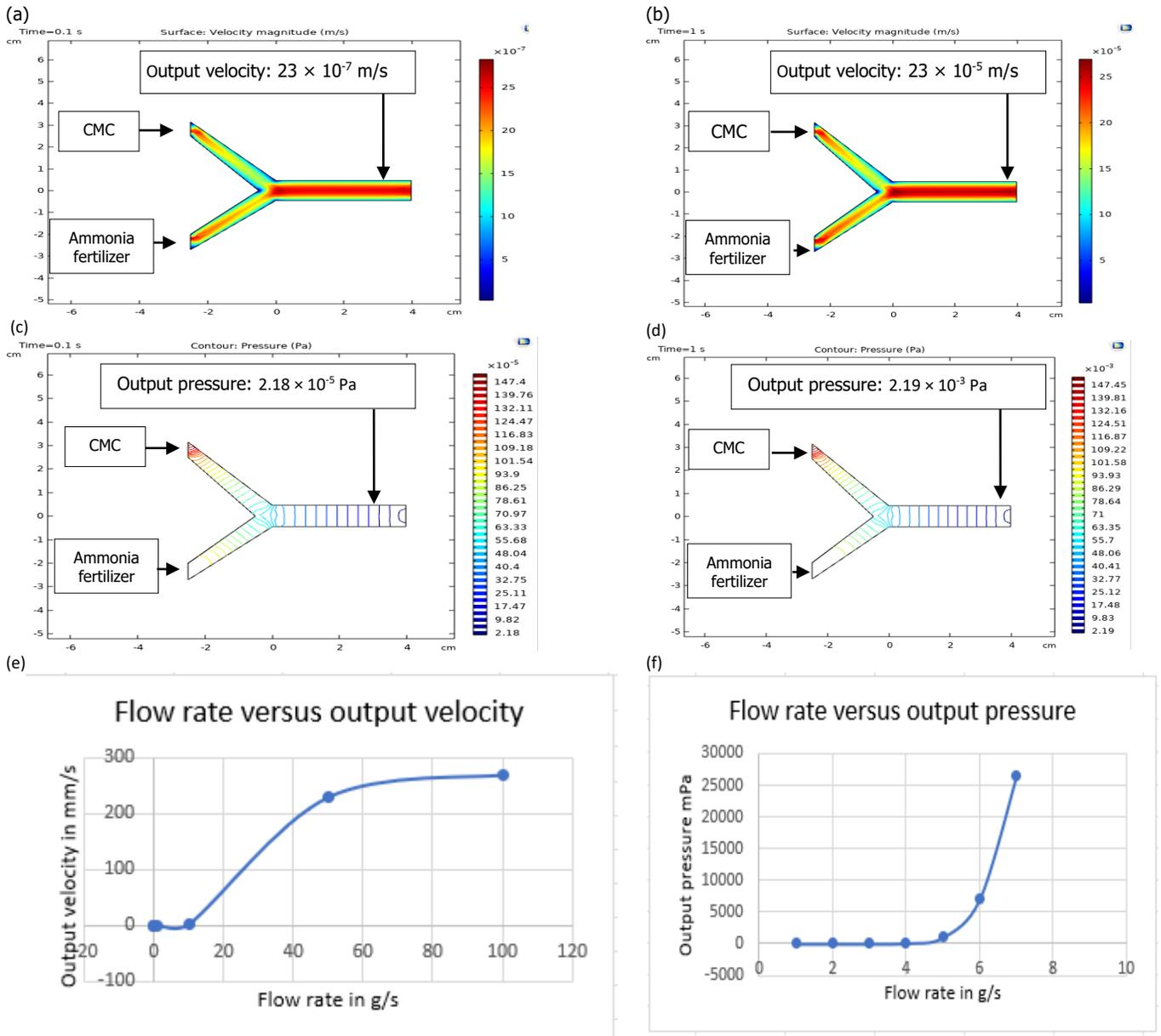
**Figure 3** Output velocity for flow rate (a) 0.001 g/s , (b) 0.1 g/s , output pressure for flow rate (c) 0.001 g/s, (d) 0.1 g/s and graph of flow rate versus (e) pressure and (f) velocity in co-axial milli-fluidic factors. Additional pressure decreases occur as a result of momentum changes in elements such as bends, compression,
