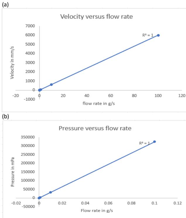
**Figure 6** Graph of (a) velocity versus flow rate and (b) pressure versus flow rate in tri-axial extruder
