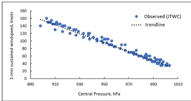
**Figure 5** Relationship of Central Pressure to Maximum Wind
