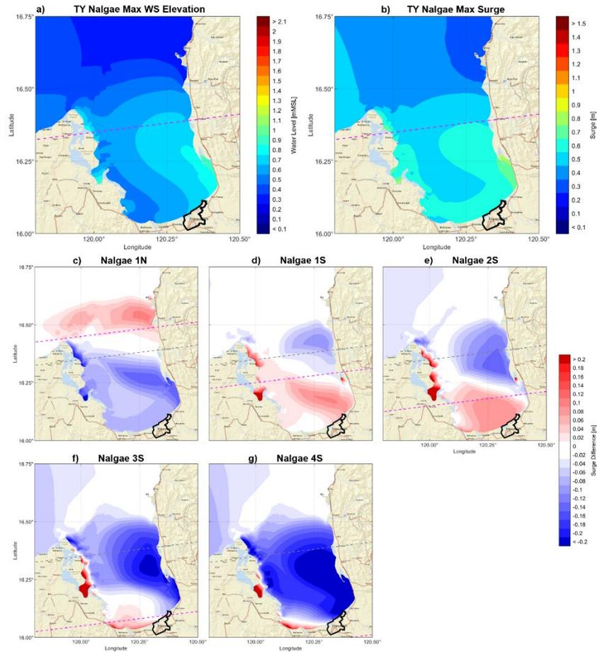
**Figure 8** Surface plots of simulated (a) maximum water surface elevation (storm tide), (b) storm surge, and (c) – (g) surge difference of synthetic tracks with respect to the original historical typhoon track of TY Nalgae 2011
