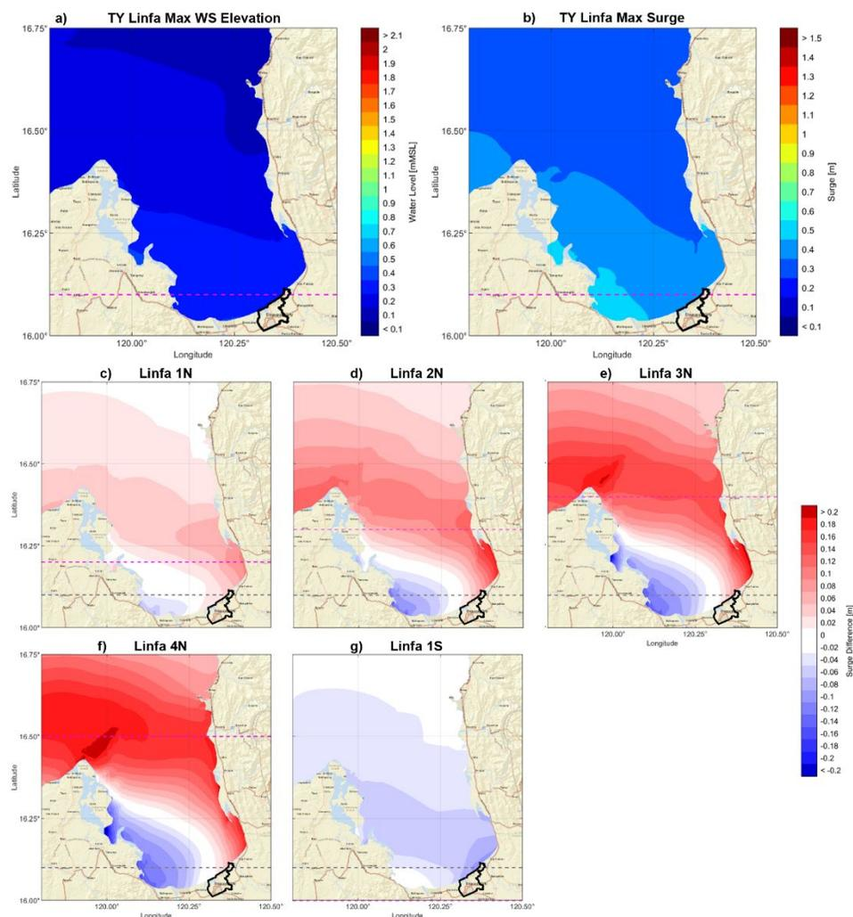
**Figure 9** Surface plots of simulated (a) maximum water surface elevation (storm tide), (b) storm surge, and (c) – (g) surge difference of synthetic tracks with respect to the original historical typhoon track of TY Linfa 2003
