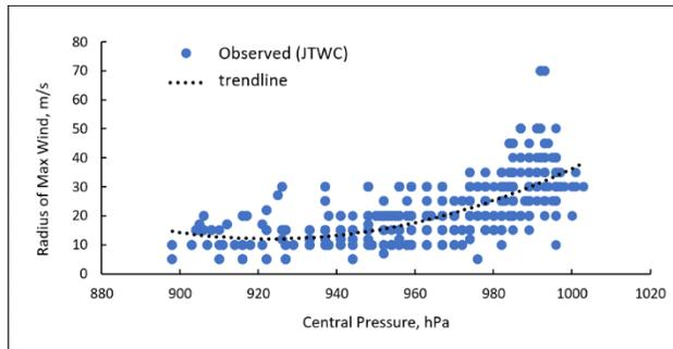
**Figure 6** Relationship of Central Pressure to Radius of Maximum Wind
