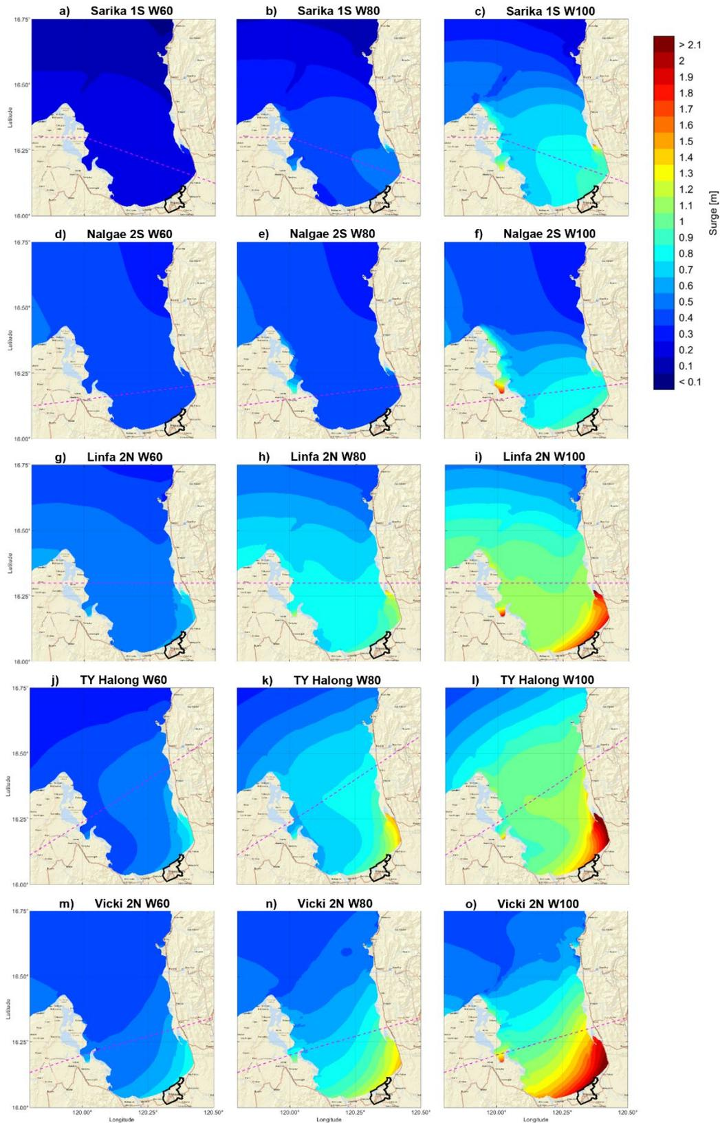
**Figure 13** Surface plots of maximum storm surges for the critical tracks with windspeeds of 60, 80, and 100 knots (a) to (o). Plots in rows are the identified critical tracks for the five historical typhoon groups. W60, W80 and W100 notations refer to windspeeds of 60, 80, 100 knots, respectively.
