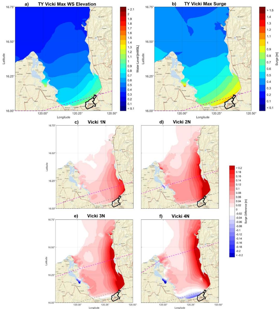
**Figure 11** Surface plots of simulated (a) maximum water surface elevation (storm tide), (b) storm surge, and (c) – (f) surge difference of synthetic tracks with respect to the original historical typhoon track of TY Vicki 1998
