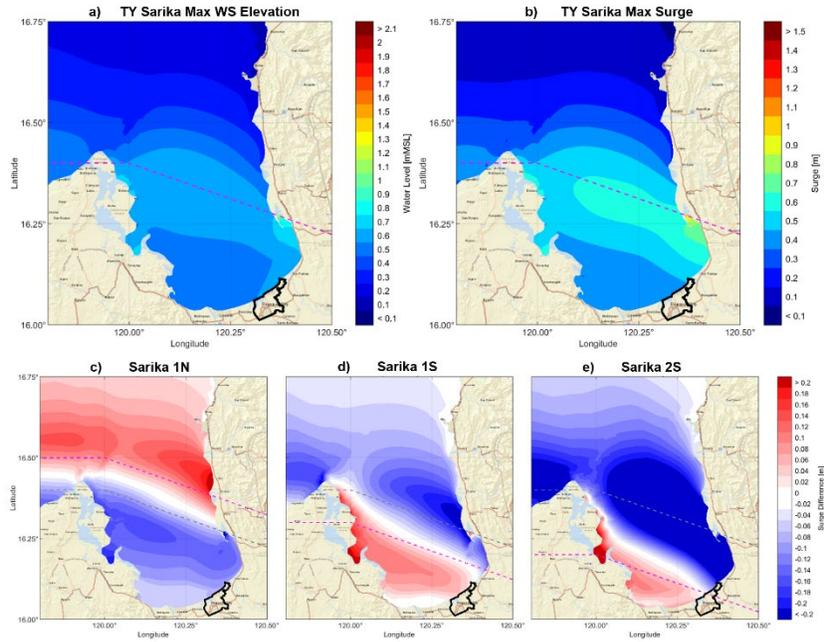
**Figure 7** Surface plots of simulated (a) maximum water surface elevation (storm tide), (b) storm surge, and (c) – (e) surge difference of synthetic tracks with respect to the original historical typhoon track of TY Sarika 2016. The pink dashed line represents the tracks used in the simulation and the gray dashed line in (c) – (e) is the track of TY Sarika. Polygon with black solid line represents the boundary of Dagupan City.
