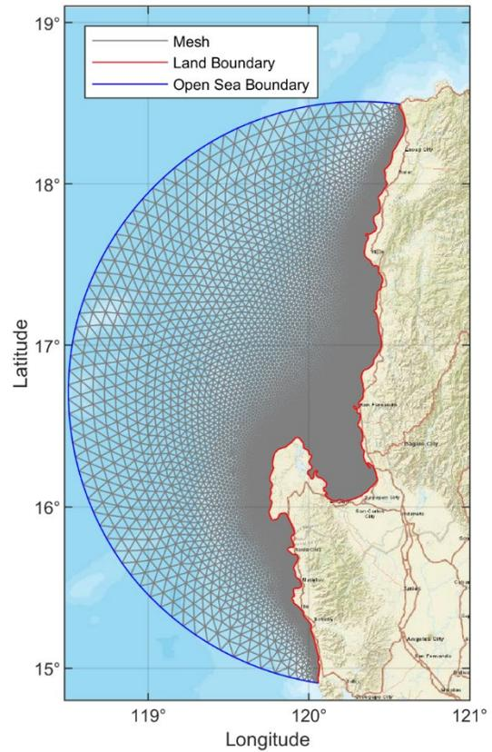
Figure 1 ADCIRC model domain and mesh of the study
