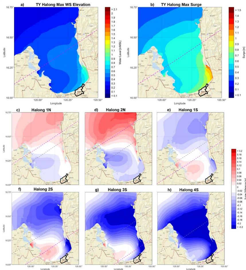
**Figure 10** Surface plots of simulated (a) maximum water surface elevation (storm tide), (b) storm surge, and (c) – (h) surge difference of synthetic tracks with respect to the original historical typhoon track of TY Halong 2008
