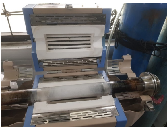
Figure 7 Exposure of MOC-3 to CO 2 gas for 7 days.
