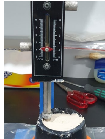
Figure 1 Vicat apparatus used for setting time test
