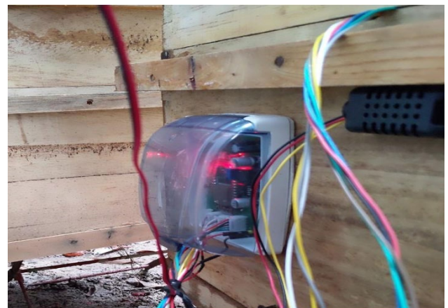
Figure 6 The IOT system for collecting the bee's sound
