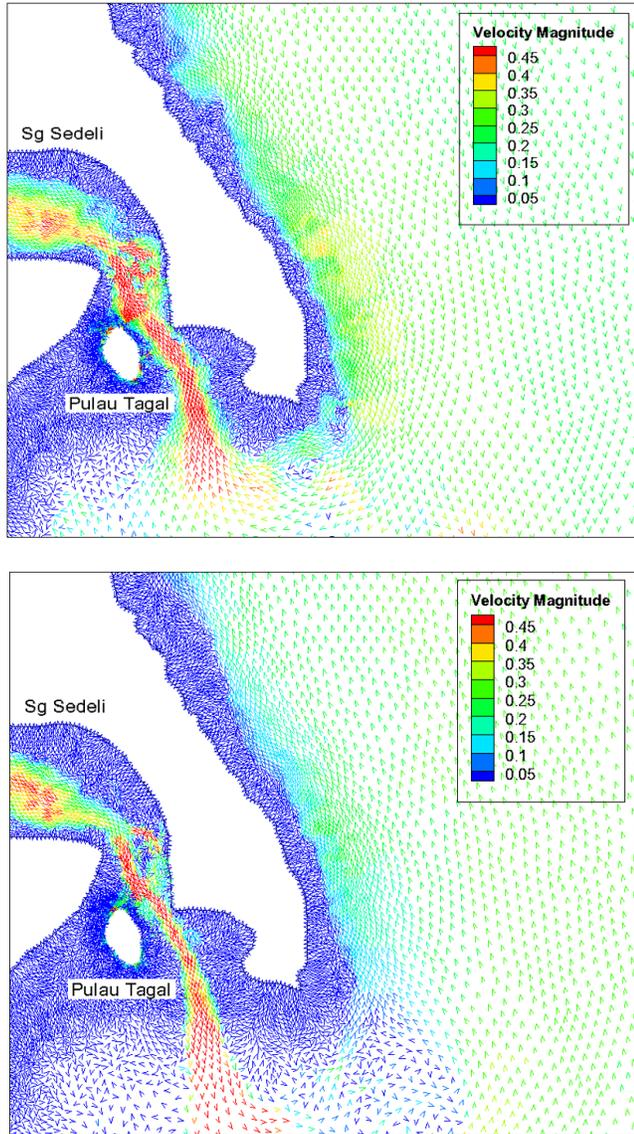
Figure 7 Current vector diagram during flood tide (top) and ebb tide (bottom)
