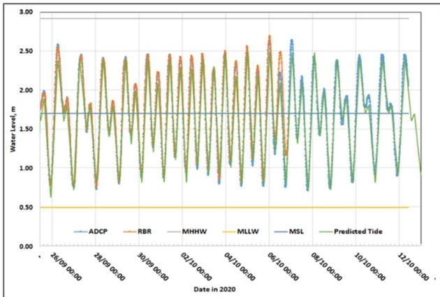
Figure 4 Comparison between measured water levels using ADCP and RBR duet and predicted tide from tide table
