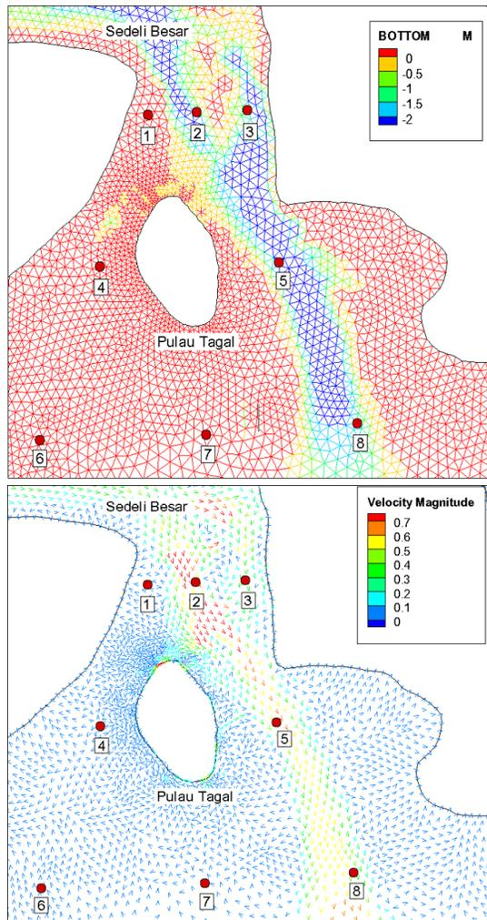
Figure 10 Bed elevation (top) and velocity (bottom) field around Pulau Tagal
