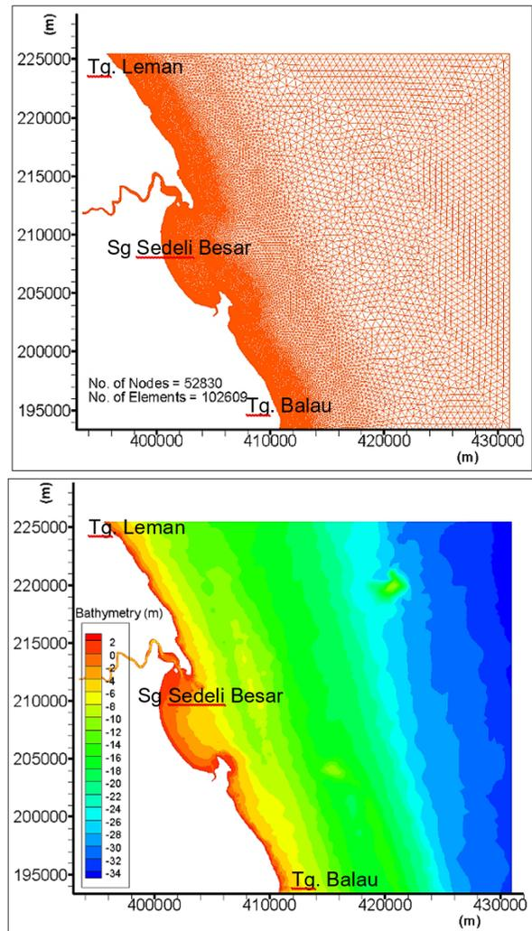
Figure 3 Model mesh (top) and bathymetry (bottom)
