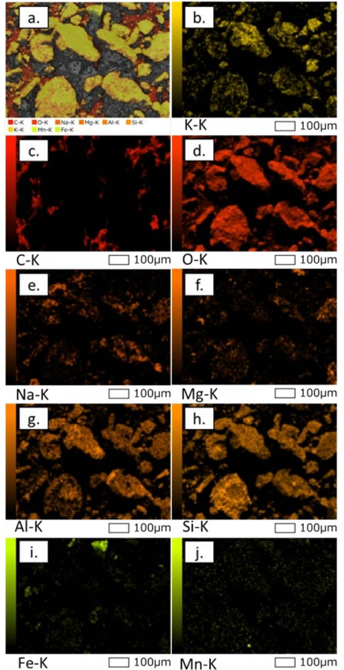
**Figure 3.** T'Boli gold tailings overall elemental mapping (a), and the corresponding specific elemental mapping of (b) K, (c) C, (d) O, (e) NA, (f) Mg, (g) Al, (h) Si, (i) Fe, and (j) Mn.
