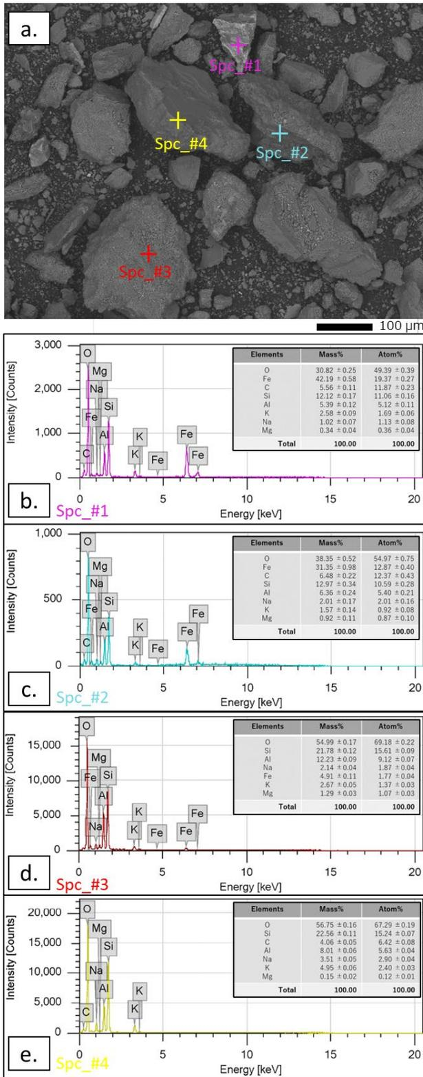
**Figure 2.** SEM-EDX spectra at different points on the surface of the T'Boli gold tailings: (a) SEM imaging of the T'Boli gold tailings, (b) spectra at point 1, (c) spectra at point 2, (d) spectra at point 3, and (e) spectra at point 4.
