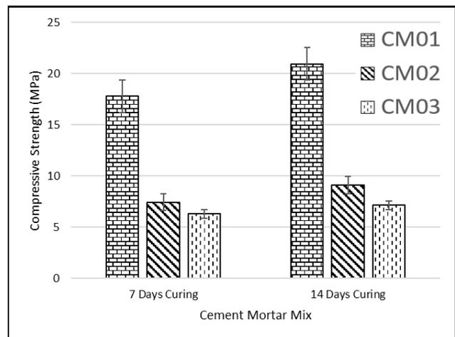
**Figure 4.** The compressive strength (MPa) of the cement mortar with different proportions of gold tailings at different curing period.
