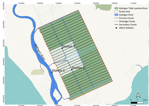
Figure 4 Study area and automatic water level recorder (AWLR) station (Base map from OSM Humanitarian Data Model, processed with QGIS 3.28.0)
