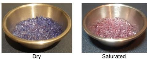
Figure 3 Silica gel saturation colors
