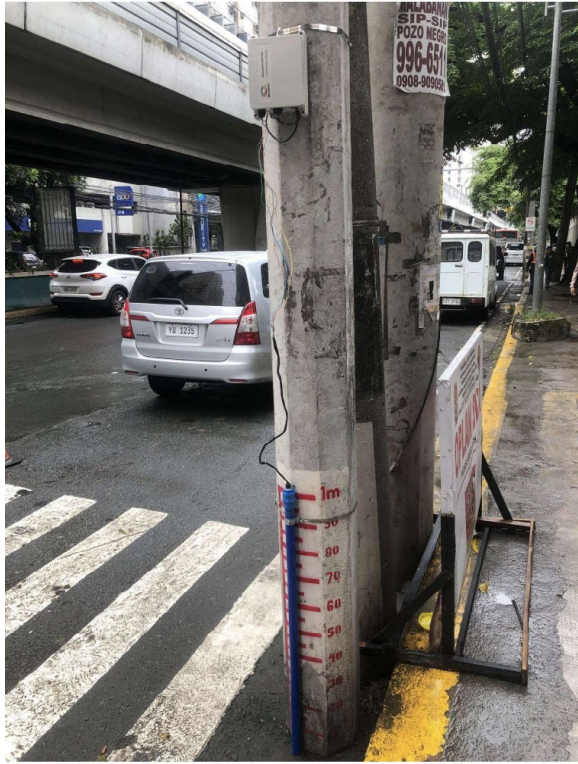
Figure 10. Image of the Overall Flood Monitoring system including the microcontroller box during field testing
