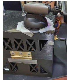
Figure 12. Attachment of Bottom Chassis and Camera Mount
