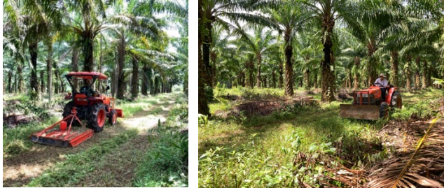
(a) Kubota L3218SP (b) Kubota L3608SP Figure 18 Kubota tractor is cutting weed while driving
