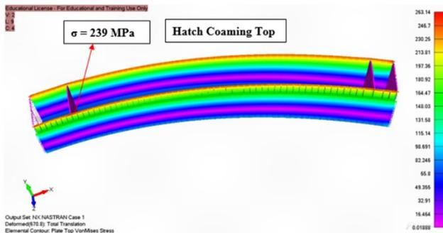
Figure 8 Hull girder stress at midship (Hogging condition)
