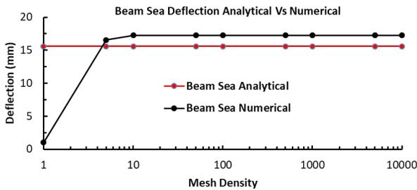
Figure 22 Comparison of Analytical vs Numerical deflection (Beam Sea)
