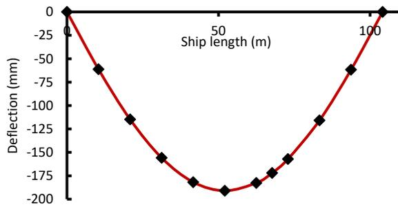
Figure 14 Longitudinal hull girder deflection along ship length (Sagging-head Sea)
