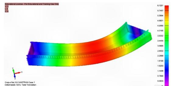
Figure 26 Transverse hull girder deflection along ship length (Beam Sea)
