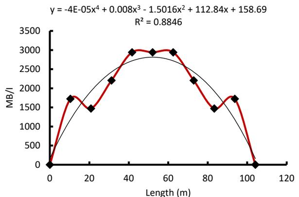
**Figure 13**  $M_B/I$  curve along ship length (Beam Sea)
