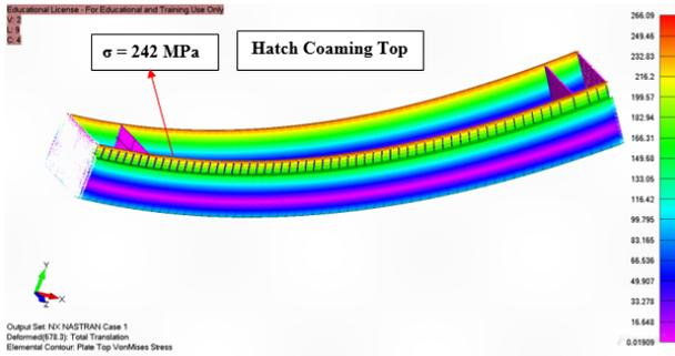
Figure 7 Hull girder stress at midship (Sagging condition)
