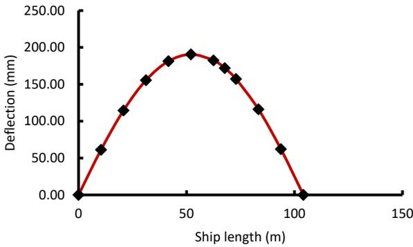
Figure 15 Longitudinal hull girder deflection along ship length (Hogging-head Sea)
