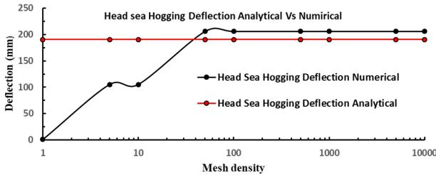
Figure 20 Comparison of Analytical vs Numerical deflection (Hogging Head Sea)
