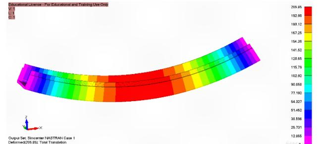
Figure 17 Longitudinal hull girder deflection along ship length (Sagging Head Sea)
