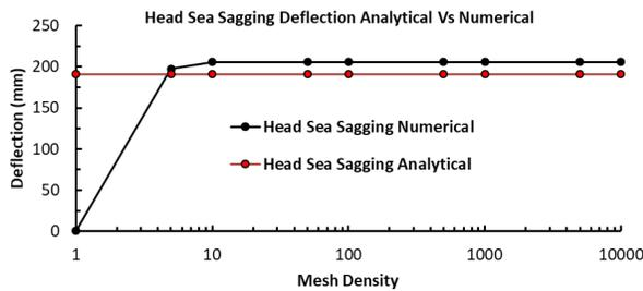
Figure 21 Comparison of Analytical vs Numerical deflection (Sagging Head Sea)
