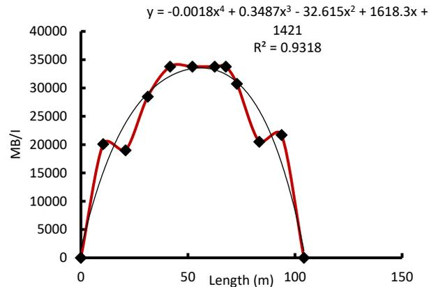
**Figure 11**  $M_B/I$  curve along ship length (Sagging-head Sea)
