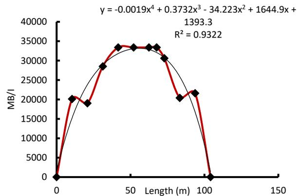
**Figure 12**  $M_B/I$  curve along ship length (Hogging-head Sea)
