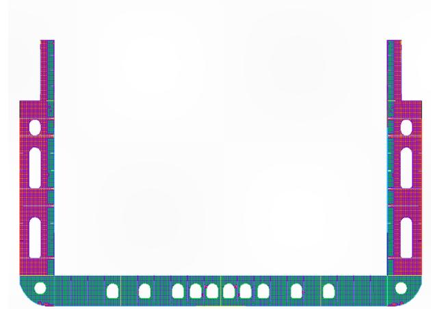
Figure 3 A typical mesh arrangement of the transverse web
