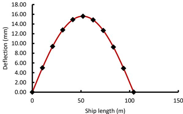
Figure 16 Transverse hull girder deflection along ship length (Beam Sea)
