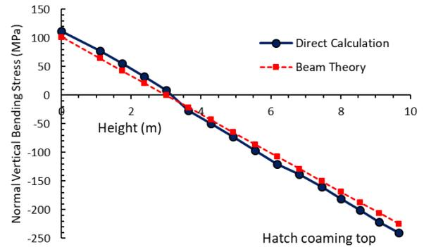
Figure 6 Comparison of hull girder stress between beam theory and direct calculation at midship (Sagging condition)
