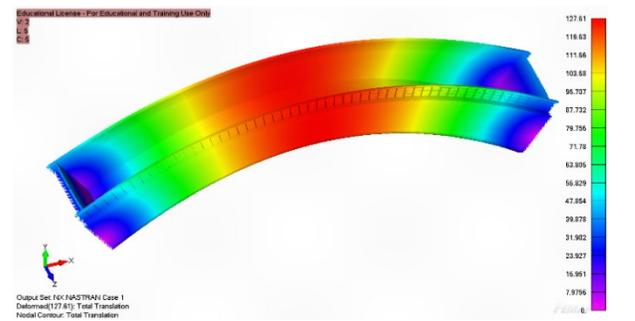
Figure 25 Longitudinal hull girder deflection along ship length (Hogging Head Sea)
