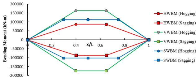
Figure 2 Comparison of the investigated ship's bending moments
