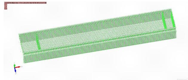
Figure 1 Generated FE model of the investigated ship in FEMAP
