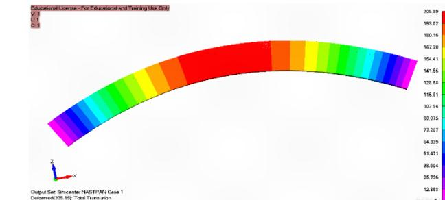
Figure 18 Longitudinal hull girder deflection along ship length (Hogging Head Sea)
