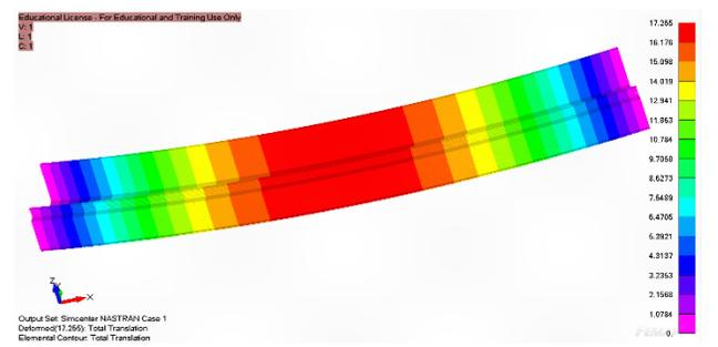
Figure 19 Transverse hull girder deflection along ship length (Beam Sea)
