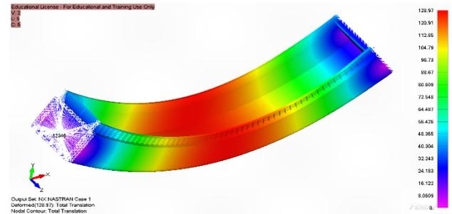
Figure 24 Longitudinal hull girder deflection along ship length (Sagging Head Sea)
