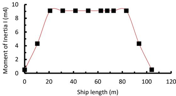
**Figure 9** Distribution of the moment of inertia (Y axis) along ship length m<sup>4</sup>
