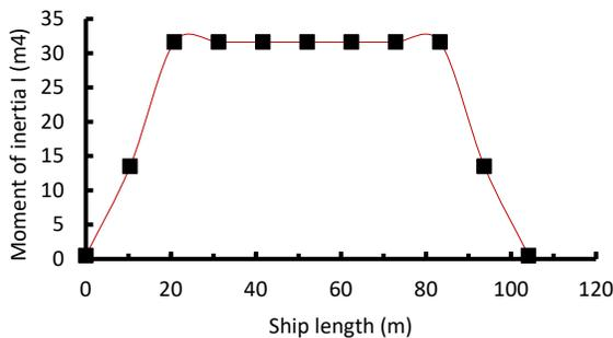
**Figure 10** Distribution of the moment of inertia (Z axis) along ship length
