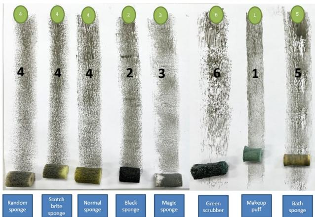
Figure 8 The foam ranking based on visual inspection
