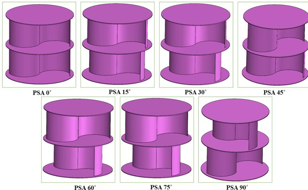
Figure 4 The design of a Savonius rotor variant.
