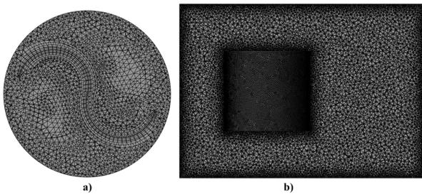
Figure 6 Meshing results in a) rotational domain and b) stationary domain
