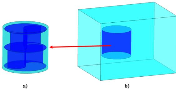
Figure 5 Domain modeling: a) rotary domain and b) stationary domain.
