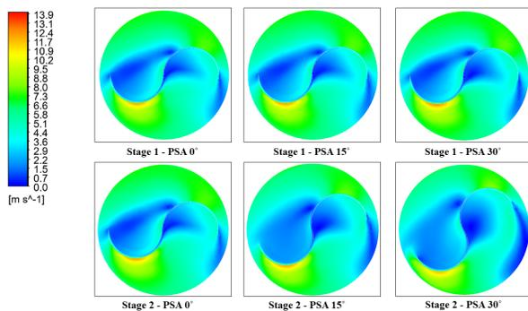
Figure 12 Velocity contours on the Savonius rotor with PSA variations.
