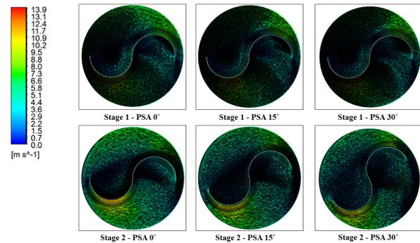
Figure 13 Vector velocity on the Savonius rotor with PSA variations.
