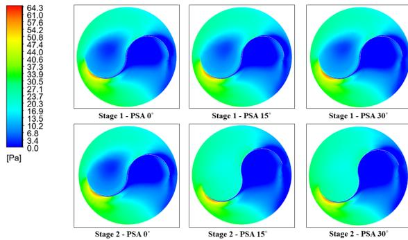
Figure 11 Pressure contours on the Savonius rotor with PSA variations.
