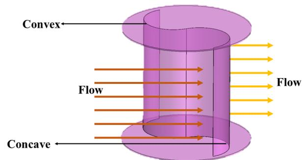
Figure 2 The functioning principle of the Savonius rotor.
