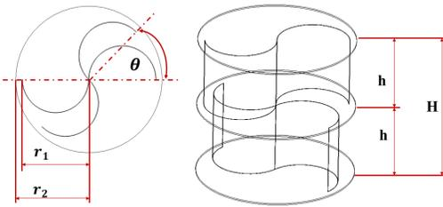
Figure 3 Rotor design dimensions.
