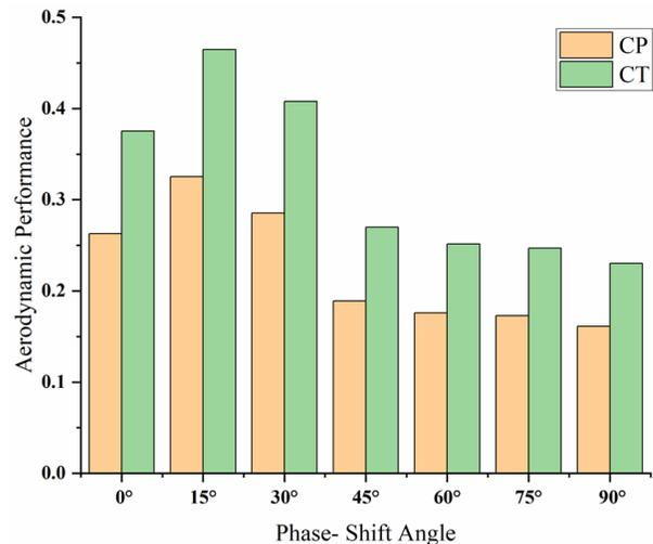
Figure 10 Aerodynamic performance results on the Savonius rotor with PSA variations.
