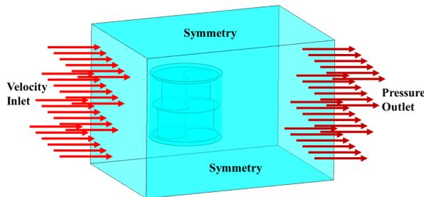
Figure 7 Savonius Turbine Modeling Schematic.
