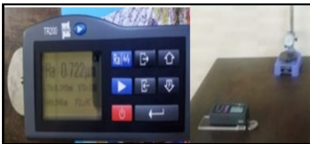
Figure 3 Surface roughness checking for substrate and coatings.
