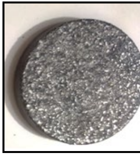
Figure 2 Tungsten Carbide coating done on substrate by Electro-Spark Deposition Method.
