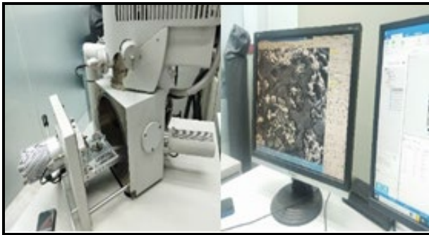
Figure 7 FESEM & EDS for substrate EN19 and Tungsten Carbide done on Quanta 200F machine.
