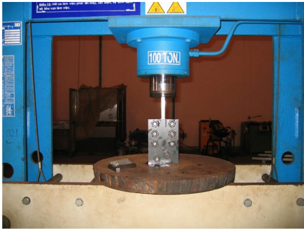
Figure 3 ECAP experiment on 100 Ton hydraulic press
