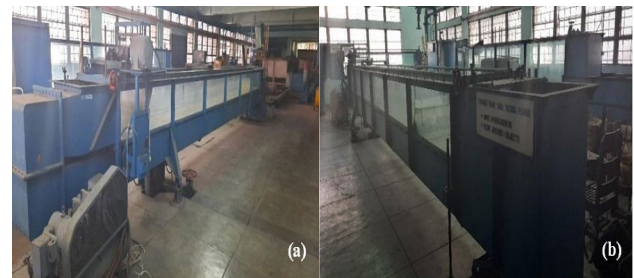
Figure 1 The existing wave flume: (a) inlet and wavemaker side and (b) outlet to sump pit below deck
