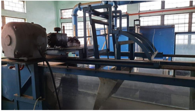
Figure 2 The existing wave generator setup consisting of the motor, connecting rod and paddle
