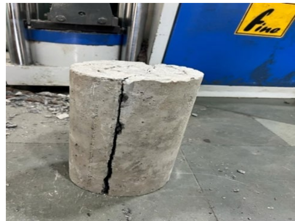
Figure 6 Crack occurred in cylinder
