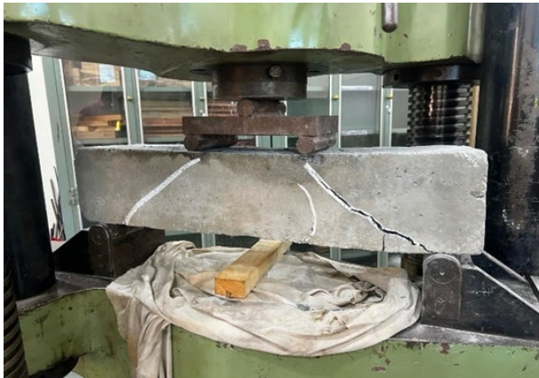
Figure 9 Crack marked on beam
