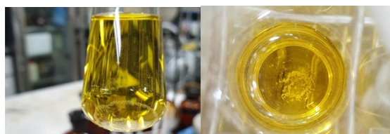
Figure 4 Precipitates were observed in the tube with (a) 1.67 g of \text{HgSO}_4 and (b) 33.3 g of \text{HgSO}_4
