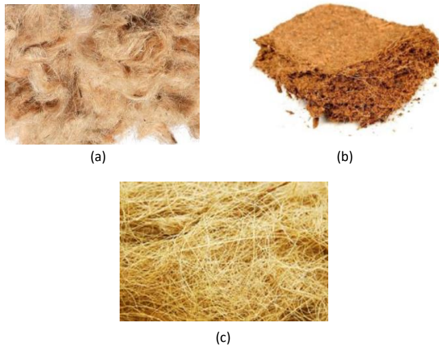
Figure 2 General overview of the structural and morphological characteristics of natural fiber specimens: (a) kenaf fibers, (b) coconut coir, and (c) palm leaf fiber.
