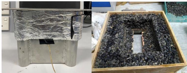
Figure 6 Overview of H-Shaped Heat Sink with Aluminium Tube as PCM Storage with Asphalt mock-up
