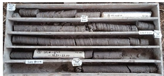
Figure 7-Photo core of claystone, claystone intercalated with sandstone-siltstone
