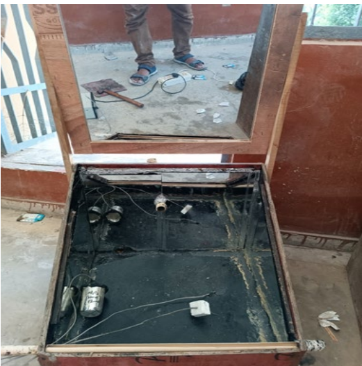
Figure 4 Solar still filled with nano fluid in Silver (Ag) cylinder
