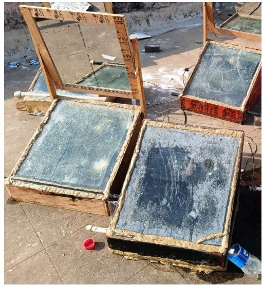
Figure 5 Conventional type single slope solar still setup
