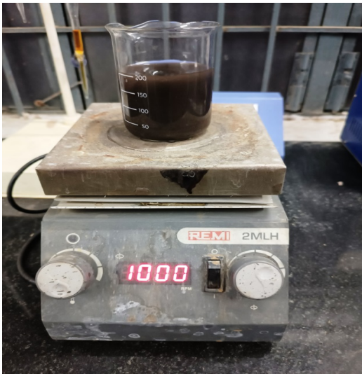
Figure 2 Mechanical mixing of CuO nano particles by mechanical stirrer
