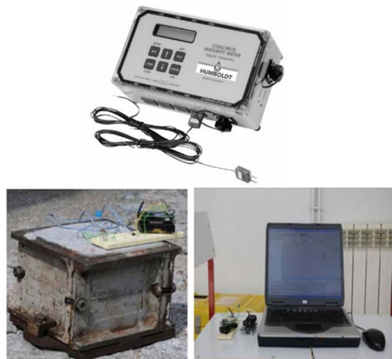
Figure 7 (a) Maturity testing equipment [69] (b) Concrete Temperature monitoring with wireless sensors [70]
