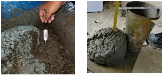
Figure 11 Measurement of slump and recording of the temperature of the mix
