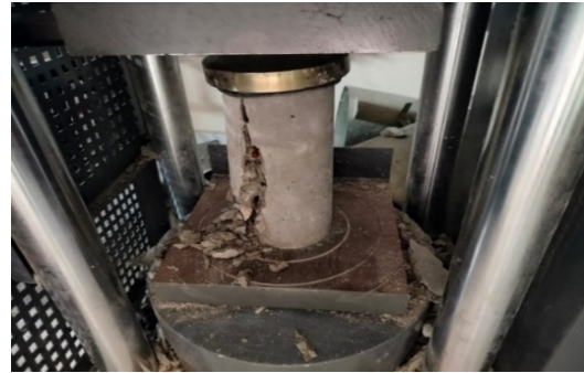
Figure 9 The load was applied to the cylindrical specimen to determine its compressive strength.
