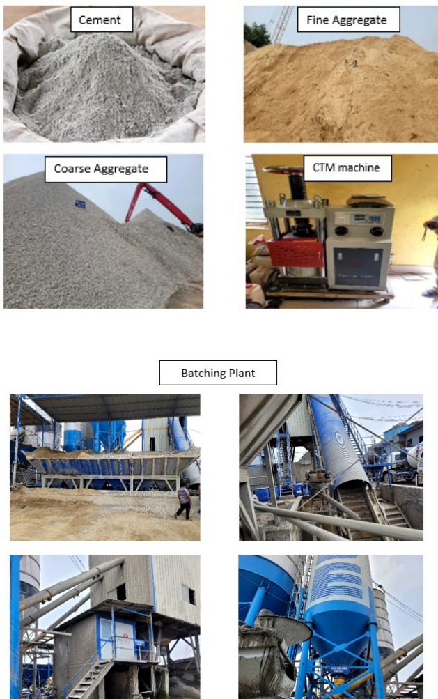
Figure 8 Materials, batching plant, and CTM machine used for concrete production
