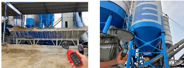
Figure 5 (a) Measuring wind velocity and air temperature using anemometer (b) Measuring relative humidity using hygrometer
