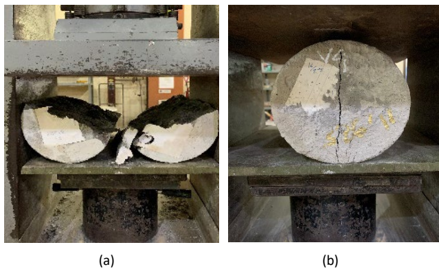
Figure 10 Failure mode of tensile splitting strength test (a) Mode A and (b) Mode B
